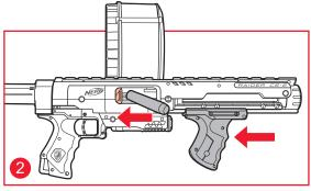
Pull Slam Fire Handle back and open Jam Clearing Door to remove jammed dart.
