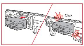
Attach Drum Connector as shown. Be sure Clip Release Button faces rear of blaster.
